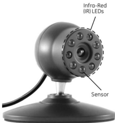
It turns on/off the Infra-Red (IR) LEDs on the front of the camera. These LEDs provide artificial light that allows the camera to 'see' in the dark. **Night Vision will appear as a Black and White image.** When the image sensor detects enough light, color will return to the images.
